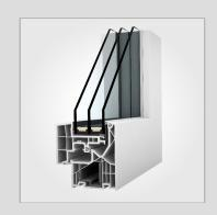
The narrow construction depth of 74 mm including aluminium cladding, and the innovative glass sash make the KF 320 a popular product. The special sash construction has the appearance of fixed glazing, but is in fact an opening window. If the frame is fully rendered, the result is an almost frameless glass architecture. I-tec Glazing ensures excellent stability, thermal insulation and security, thanks to all-round bonding of the glass pane. Also available as a uPVC only window.
